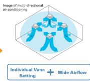
The combination of individual vane setting. which enables the optimal outlet setting for each room layout, and the wide airflow function works to ensure even temperature distribution throughout each room. The result is uniformly comfortable air conditioning
